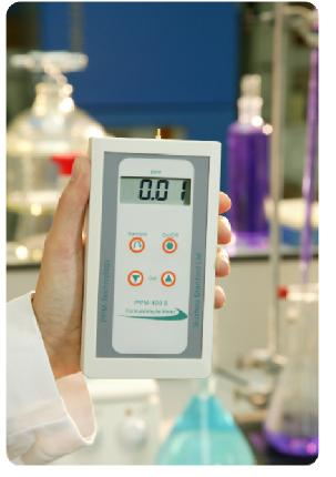
The PPM-400ST is the latest 3-parameter instrument from PPM Technology, which directly measures airborne formaldehyde concentrations as well as ambient temperature and humidity levels. It can accurately measure low levels of formaldehyde, even in humid conditions using unique compensation techniques, while still maintaining ease of use and simple calibration.
