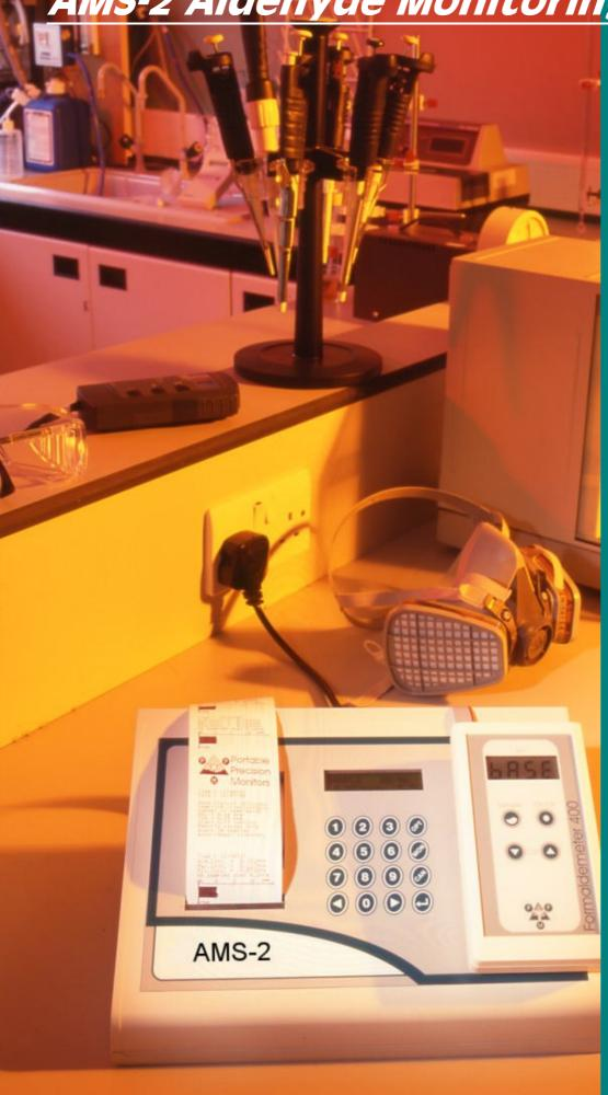
The ultimate datalogging gas detection system for formaldehyde and glutaraldehyde from PPM Technology
